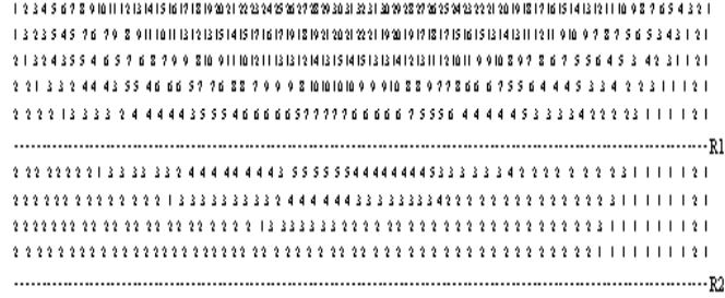
Fig.4(a) - The Wallace tree structure for a 32-bit multiplier
