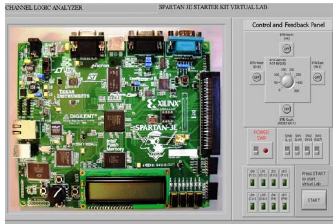
Fig. 2. the GUI showing the FPGA development board and the I/O Control and Feedback Panel.
