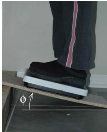
Figure 4: Bathroom scale used in a vector decomposition activity.
